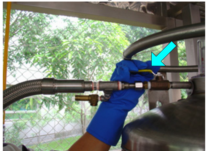
(6) Make sure the residual pressure is less than 0.5bar, then open the refilling valve.
